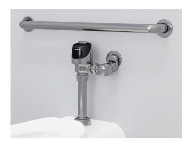
Sloan's new Offset Adapter for G2, SOLIS®, and ECOS® Flushometers helps keep your facilities accessible. This unassuming adapter creates enough space for an ADA-compliant grab bar by lowering the total height of the flushometer by 1-1/2 inches without having to relocate the water supply inlet pipe. It's a simple update that saves your facility from the costs and complexities of opening walls or workarounds like split grab bars.
